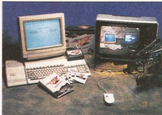
DCTV is another solution to the problem of insufficient colour resolution. It plugs in externally to give a composite video signal with thousands of colours.
